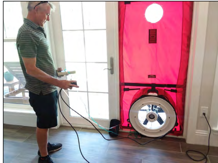
A building air leakage test underway.
